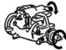
REVERSE ROTATION Rotate old unit input shaft clockwise, output shaft will rotate counter-clockwise
